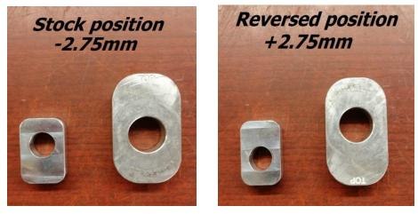
**After installation, check chain slack!** The stock OEM reference for chain slack is only good for the stock shock length and the stock swingarm pivot height. If you increase shock length everytime you change pivot position you have to check for chain binding.
