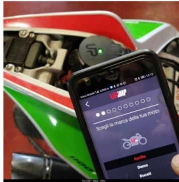
Download the App on your phone then connect the T800+ to the bike diagnostic port using the supplied cable. 2009-20 cable, identified as "MARELLI", fit the flat black diag port under passenger seat plus has a fused +12volt feed for battery connection. The 21+ cable, named "EURO5a", plugs in the red square diag port under the rider seat. Pics of the connections are in the **NOTE C**).
